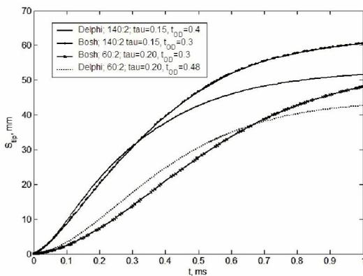
Fig. 3. Spray tip penetration for Delphi and Bosch injectors; ambient pressure 2 MPa; injection pressure 60 MPa ( $\beta = 1.6$ ) and 140 MPa ( $\beta = 1.3$ )
