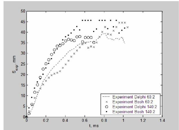
Fig. 1. Comparison between Bosch and Delphi spray tip penetration experiments; ambient pressure 2 MPa; injection pressure 60 MPa and 140 MPa
